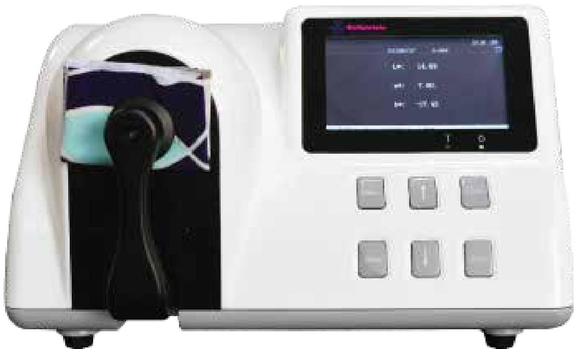
**Spectro-9801** is a high performance spectrophotometer with sideward test aperture. It could be widely used for printing, textile, plastic, food, medicine, automobile industries to meet customers' color measurement requirement.
